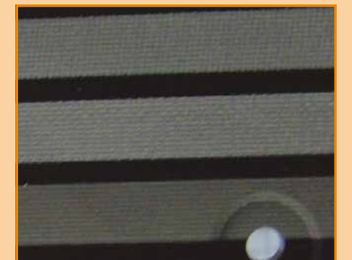
Three different roughnesses on a POM casing. The parameters can be simply changed via the software.
