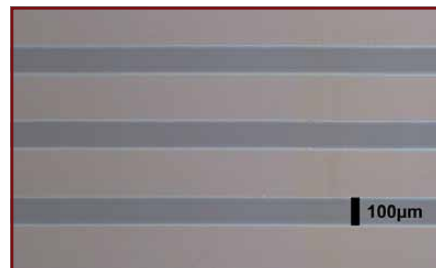
Fig. 2, 100 µm scribes through ITO (P1)
