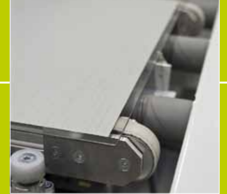
Thin-film solar module with 4JET laser edge deletion
