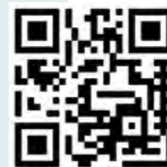
QR Code with 11 alphanumeric characters Level H (highest) error correction
