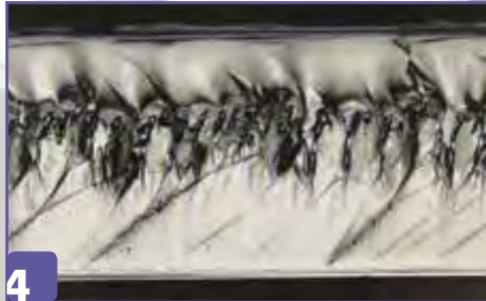
Microscopic images of the cut edges with various process parameters (Gorilla® glass)
