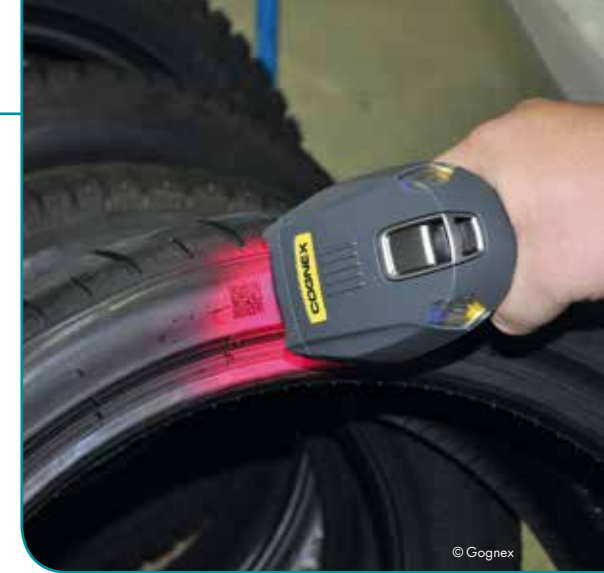
Identification at the touch of a button: Handheld readers of the DataMan 8000 series by Cognex detect and read 2-D codes quickly and reliably
