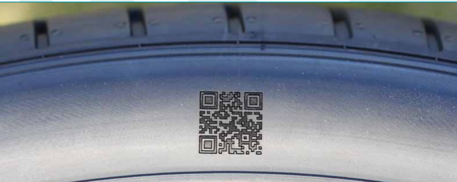
Laser Engraving on a tire sidewall
