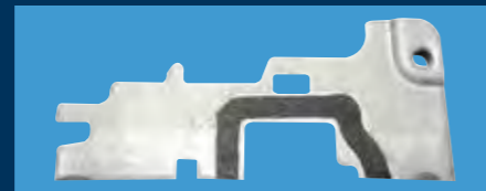
Adhesion improvement by laser preparation
